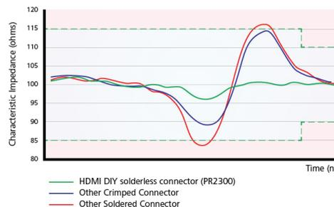
Our crimp connector has better impedance response than most other connectors – near 100 Ohm impedance!
